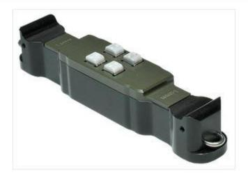
Two row fixed space transducer modules with four transducers per module to inspect at a high frequency range, which increases sensitivity to small local defects (pits) while decreasing sensitivity to supports and erosion. These modules require the G4 Mini (Fully Loaded) or the Wavemaker® G4 with the MF option. Key application areas include:
