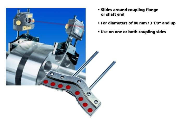
Shafts can't be rotated? No problem! This bracket allows measurement and alignment to be performed when one or both shafts cannot be rotated. The magnetic sliding bracket is placed upon the back of the coupling or front corner of the uncoupled shaft and slid around from one measurement position to the next. Suitable for shaft/coupling diameters from approx. 80 mm (3 1/8") on up.
